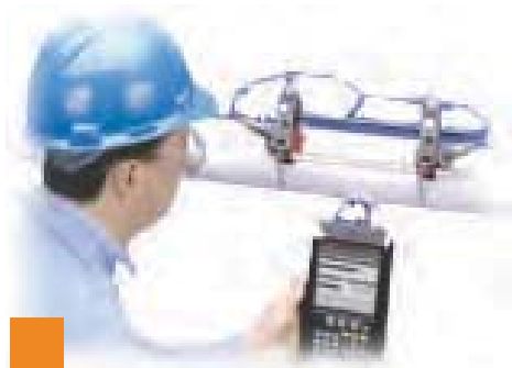
Ultrasonic Flow measurement System Pnametrics, mod PT878 for Liquids Laser Ailignment System Go Fixture
